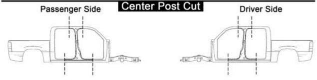
Standard Post Cut = 6 inches both directions at top post, halfway through each bottom door opening.
